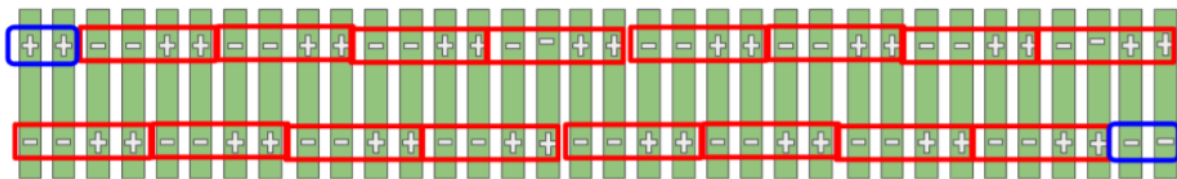
Figure 29: 2p17s Stack Configuration (Busbar Schematic)
